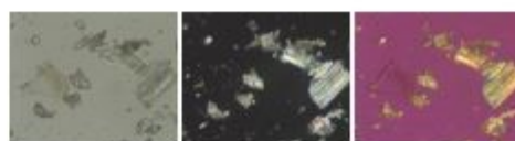
Figure 2. PLM images of Bedaquiline benzoate. Left to right: plane polarized light, cross-polarized light, cross-polarized light with red compensator
